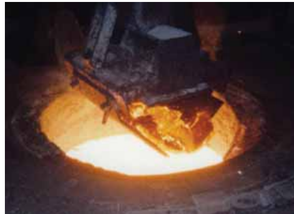
Figure 2 FERROGEN and SLAX* application helps in the removal of slag
