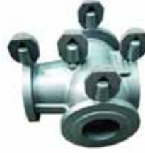
Figure 7 Casting with VS spot feeding on a twin flange section
