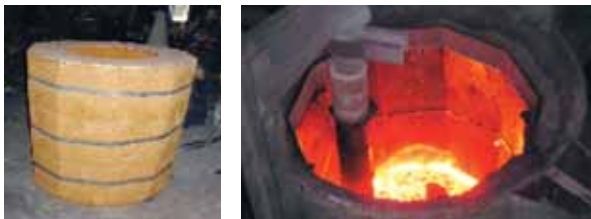
Figure 3 Ladles from 2 tonnes to 20 tonnes are lined with KALTEK. Ladle drying and preheating has been eliminated. Lower tapping temperatures are achieved with large ladles
