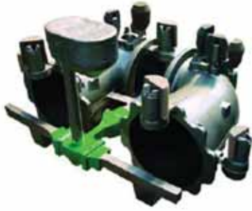
Figure 6 Casting spray with SEDEX filter (green), KALMINEX 2000 insert sleeves and FEEDEX VS spot feeding technology
