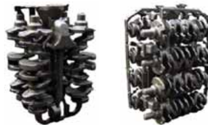
Figure 5 Original 4 cavity spray with double sand feeders and the improved 8 cavity spray with castings turned through 90°, doubling productivity
