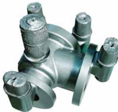
Figure 9 Using KALPUR the yield is 56%
