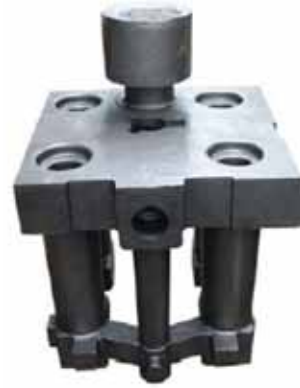
Figure 8 Finished casting: 86% yield
