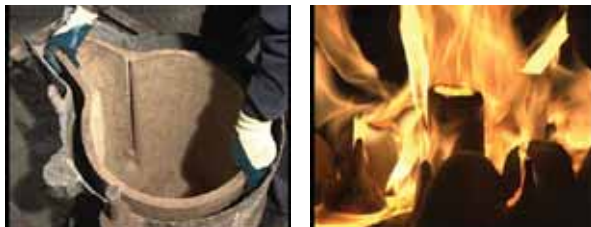
Figure 4 The ladle is not dried or preheated before use. The metal is poured at 1350 - 1380 °C with KALTEK.
