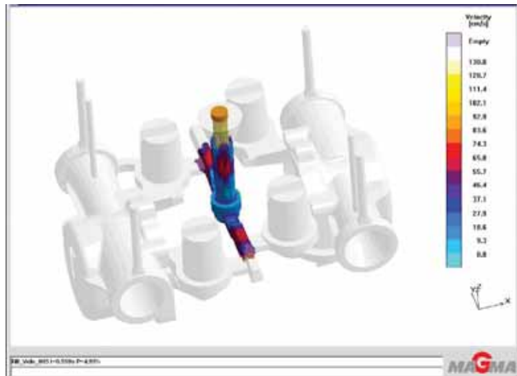
Figure 2 Simulation of a gunmetal casting ( after feeding system optimization)
